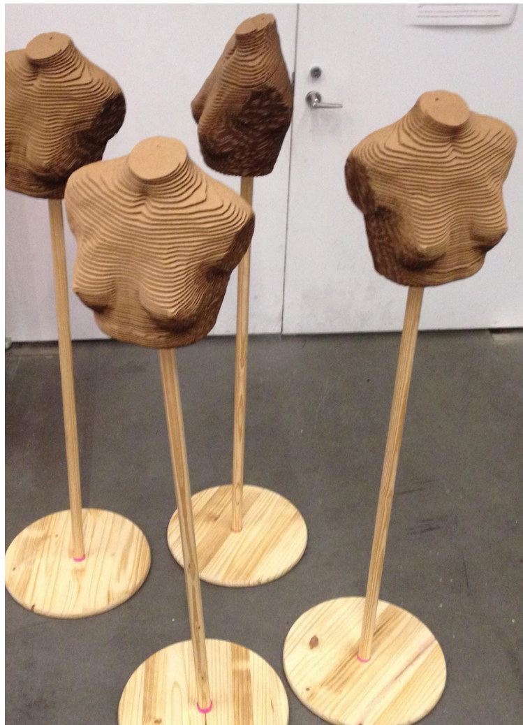
Ada Mannequin FabTextiles, Fab11, 2015 Stack slices, laser cut
