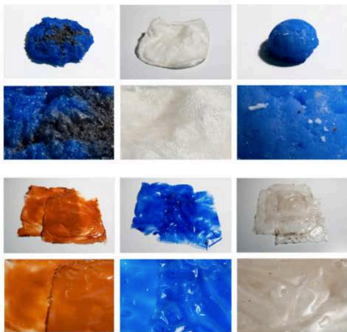
Basic recipe blue pig. more agar microwaved. Basic recipe ocre powder. Basic recipe agar agar microwaved. Basic recipe Blue pigment. Basic recipe blue pigment. Basic recipe pumice powder.
